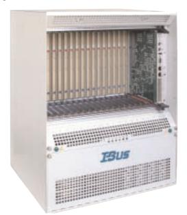
The C1221 is the first I-Bus enclosure to support up to 20x IBC2802 CPU boards
